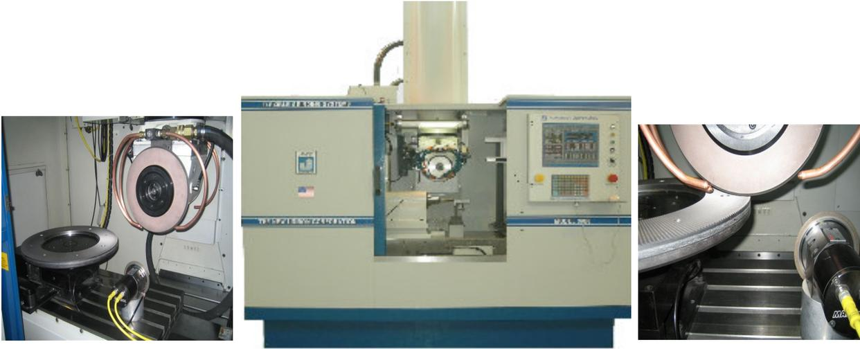
Unison's Model 9100 Pulverizer Blade Regrinder is a 5-Axis turnkey grinder featuring an integrated 25 horsepower, direct drive, dual ended spindle. The direct drive spindle motor provides a continuous torque rating through its entire operating range.
