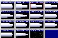
The Model 2150<sup>™</sup> has the ability to dress grinding wheels in cycle with automatic size compensation for wheel wear after dress. Whether dressing a simple flat wheel or an intricate profile, dressing can be automatically executed during grind cycles as controlled by the machine's operator.
