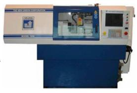
The Model 1500 is a rigid production grinding system designed to grind round & non-round OD shapes, as well as contours and peel grinding. Featuring Unison's proprietary grinding technology, the Model 1500 is capable of meeting the most demanding grinding applications with fast cycle times.
