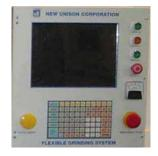
The UPC utilizes the Windows 7™ Operating System and the software monitors all critical machine functions and alerts the operator to problems encountered during grinding. Errors are tracked and logged within the machine's control to easily identify a problem. The Model 1500 can be networked and monitored via the internet or through a central data collection point.
